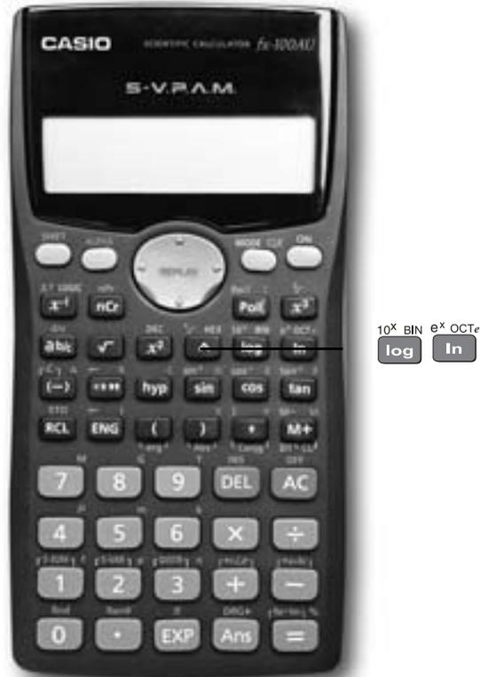
The 'log' key uses base 10 and the 'ln' key uses base  $e$  (natural logarithm).
