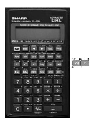
The 'log' key uses base 10 and the 'ln' key uses base e (natural logarithm).
