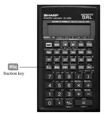
On the  $a\frac{b}{c}$  key the 'a' represents the whole part of a mixed number and the ' $\frac{b}{c}$ ' represents the fraction part of a mixed number.
