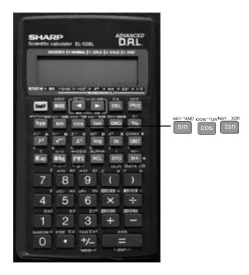
**Important**: Make sure that your calculator is in the correct mode. For example, if your calculator has RAD or GRAD on the display and you wish to work in degrees, press the DRG key until the display shows DEG.
