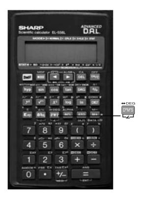
This key can be used for problems involving degrees, minutes and seconds or hours, minutes and seconds.
