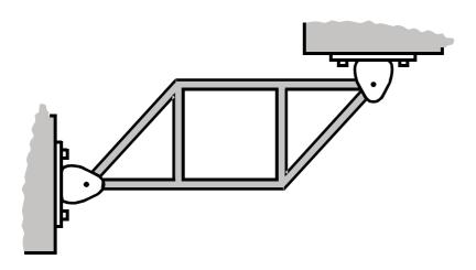
We are not going to study forces but for every joint in the truss two equations are generated, which gives us a total of 12 simultaneous equations with 12 variables. This information can be put into a  $12 \times 12$  matrix.
